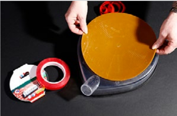
The Sealing Disc connects to the WSR using heavy duty mounting tape.
