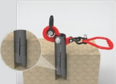
Apply force to the lifting ring, the cam will slide the mandrel causing it to expand and grip the concrete to pick up the slab
