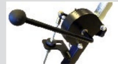
Unique blade guard design ensures safe blade coverage plus provides the dynamic directional point for cutting products so they can be controlled and removed.
