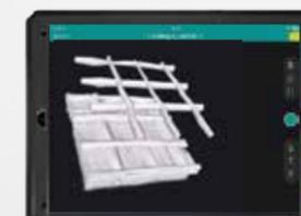
The Proceq GPR Live also has a 3D view to enable users to understand the scanned underground structure easily and more intuitively.
