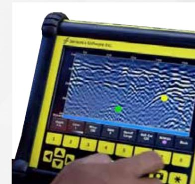
Classify targets in real time with field interpretations. Use the touch screen to colour code each target as it is located
