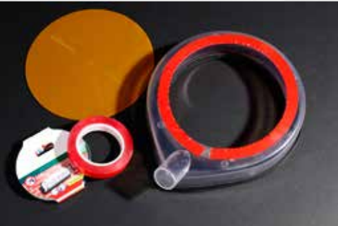
Sealing Discs are attached to the Water Slurry Rings using heavy duty mounting tape
