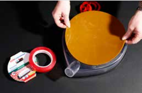
Sealing Discs are attached to the Water Slurry Rings using heavy duty mounting tape
