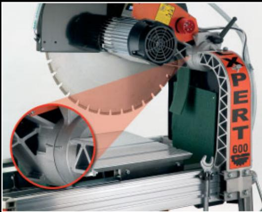
The cutting head and the arm are in die-casting aluminium to get the maximum of rigidity and lightness.
