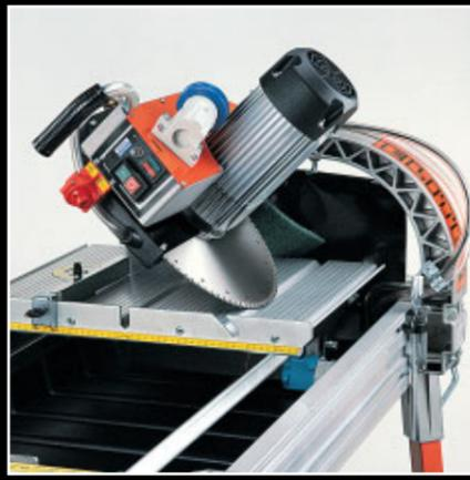
Position 45° angle cuts with relative tilting of the cutting head.
