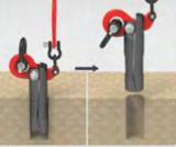
When finished, pull up release lever to easily remove the Monkey Fist from the slab
