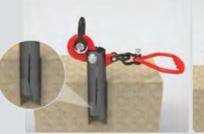
Apply force to the lifting ring, the cam will slide the mandrel causing it to expand and grip the concrete to pick up the slab
