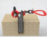
Insert the Monkey Fist into a 52 mm core drilled hole centered on the slab to be removed.
