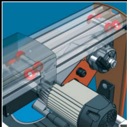
The carriage engine group slides on the rail by means 8 ball-bearings, of which 4 works always in perpendicular way respect to the rail. So doing the sliding is very fast and precise.
